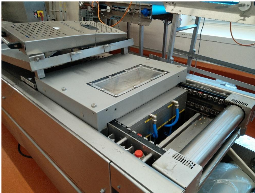
Figure 3: Matrix preheating integrated into WEBOMATIC thermoforming machine at Bedford
