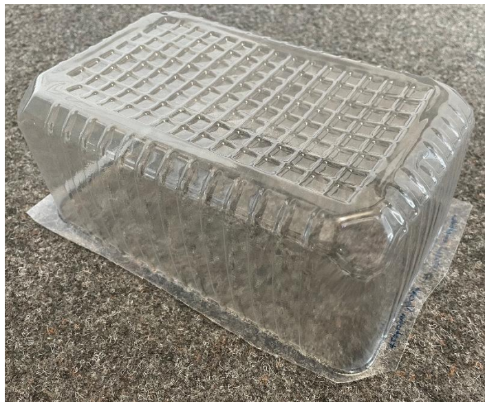
Figure 2: Molded bottom film of the optimized packaging with a film thickness of 450 µm
